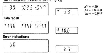
Battery power is almost exhausted. Replace battery.
