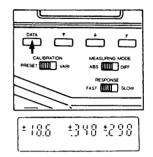
11. To store the values for Yxy in memory and complete calibration, slide the CALIBRATION selector switch from VARI. to PRESET (if not already at PRESET), press and hold F, then slide the switch back to VARI. The external display will read "CAL" for a moment as the Yxy values are stored and the meter automatically adjusts its calibration. It will then revert to the Yxy values. Calibration is now complete. The stored calibration data will remain in memory until changed or cleared by the user.
