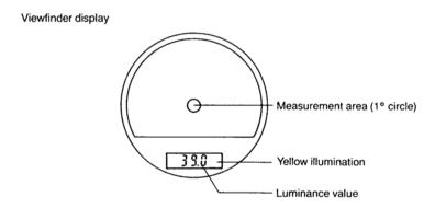
The measurement area and measured luminance value can be simultaneously confirmed in the viewfinder as shown in the figure above. The display is a digital liquid-crystal display (LCD) illuminated with a yellow LED.
