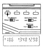
12. To store the values for Yxy in memory and complete calibration, slide the CALIBRATION selector switch from VARI. to PRESET (if not already set at PRESET), press and hold \_\_F\_\_\_, then slide the switch back to VARI. The display will read "CAL" for a moment as the Yxy values are stored and the meter automatically adjusts its calibration, then revert to the Yxy values. Calibration is now complete. The stored calibration data will remain in memory until changed or cleared by the user.
