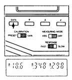
9. To store the values set for Yxy, slide the MEASURING MODE selector switch from DIFF. to ABS. Press and hold F, and slide the switch back to DIFF. The display will read "CAL" for a moment as the reference values are stored, then revert to the previous display. The stores data will remain in memory until cleared or changed by user.
