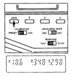
9. To store the values set for Yxy, slide the MEASURING MODE selector switch from DIFF. to ABS. Press and hold F, and slide the switch back to DIFF. The external display will read "CAL" for a moment as the target values are stored, then revert to the previous display. The stored data will remain in memory until changed or cleared by user.
