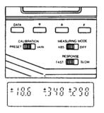
12. To store the values for Yxy in memory and complete calibration, slide the CALIBRATION selector switch from VARI. to PRESET (if not set to PRESET in step 2), press and hold F, then slide the switch back to VARI. The external display will read "CAL" for a moment as the Yxy values are stored and the meter automatically adjusts its calibration, then the display will revert to the Yxy values.
