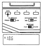
Set Y value (0.01 to 999000) by pressing and holding F and pressing either or until the displayed value matches the value displayed in step 4.
