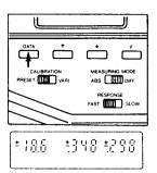
8. Slide the MEASURING MODE selector switch to ABS.
