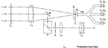
$L_2$ Objective lens L3 . L4 Eyepiece lens system М Total-reflection mirror Sı Aperture stop S2 Field stop Р Porro prism G Focusing screen Chopper F<sub>1</sub>, F<sub>2</sub>, F<sub>3</sub> Spectral-response correction filters Optical fiber cable D<sub>1</sub>, D<sub>2</sub>, D<sub>3</sub> Silicon photocells
