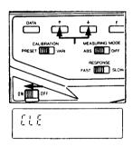
2. While pressing F, slide the CALIBRATION selector switch from **PRESET** to **VARI**. "Yxy" will appear in the external display. All values of target color and user's calibration data will be set to 0 and measurements taken at **PRESET** and **VARI**. calibration setting will be equal.
