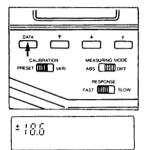
Set Y by pressing and holding F and pressing either or until the displayed value is equal to the desired value.
