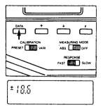
Set Y by pressing and holding F and pressing either ↑ or ↓ until the displayed value is equal to the desired value.
