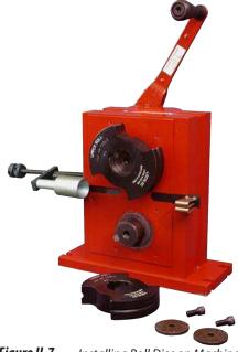
Figure II-7 Installing Roll Dies on Machine
