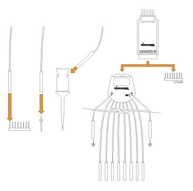
Connect the ground lead or leads to the circuit ground.
