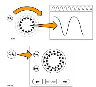
3. Examine the zoomed view of the waveform that appears on the larger, lower portion of the display. The upper portion of the display will show the position and size of the zoomed portion in the waveform, within the context of the overall record.
