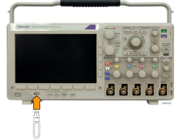
**4.** Power on the oscilloscope. The instrument automatically recognizes the replacement firmware and installs it.
