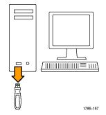
Unzip the files and copy the firmware.img file into the root folder of a USB flash drive.
