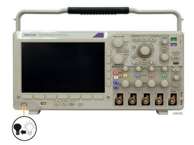
**3.** Insert the USB flash drive into the front-panel USB port on your oscilloscope.
