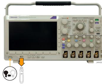
6. Power on the oscilloscope. 100 0\_\_\_ -0 2410-008 7. Push Utility. Utility 00 2410-017 Utility Page 8. Push Utility Page. 8 9. Turn multipurpose knob a and select Config. Config Set Date & Time Utility Page 10. Push About. The oscilloscope displays the Language TekSecure About firmware version number. English Erase Config Memory **11.** Confirm that the version number matches that of the new firmware. 10
