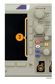
To remove a side-bezel menu, push the lower-bezel button again or push Menu Off.
