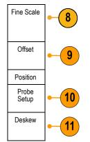
9. Select Offset to enable multipurpose knob a to make vertical offset adjustments.
