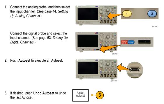
You can also disable the Autoset function if you want to set up a waveform manually. To disable or enable the Autoset function:
