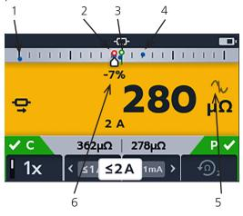
DLRO2 color display with new Difference Meter Key to Difference Meter screen:
