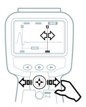
The range is set using the four way switch; press up to increase the range and down to reduce the range.
