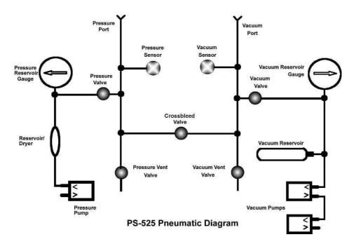
When the operator wishes to simulate an altitude, the Crossbleed, Vacuum, and Vacuum Vent valves are gently closed. The vacuum pump is then energized until sufficient vacuum is in the reservoir, as indicated on the Vacuum Reservoir Gauge. How much vacuum will be needed depends on the desired altitude, and is also affected by how long the tubing and lines are between the test box and the altimeter. **The vacuum and**
