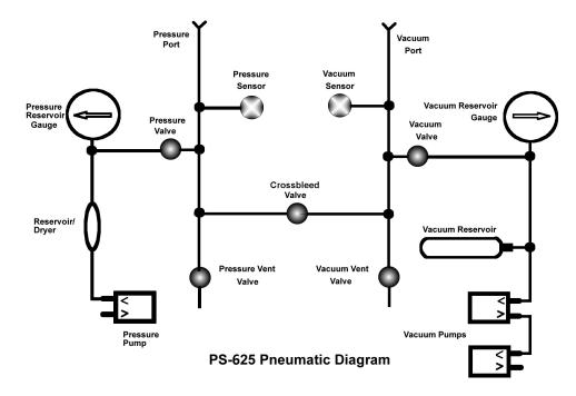
When the operator wishes to simulate an altitude, the Crossbleed, Vacuum, and Vacuum Vent valves are gently closed. The vacuum pump is then energized until sufficient vacuum is in the reservoir, as indicated on the Vacuum Reservoir Gauge. How much vacuum will be needed depends on the desired altitude and is also affected by how long the tubing and lines are between
