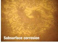
MOI 308/7 image of a small corrosion pit (dark area in the center of the picture). Corrosion is irregular in shape and can be most easily identified by moving the imager across the area being inspected. Corrosion is seen as irregular shadow shapes moving with the imager.
