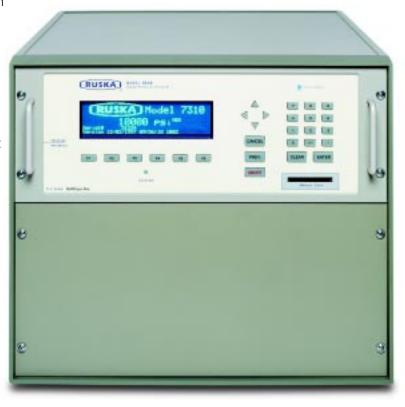
The Model 7610 High Pressure Hydraulic Controller features multimedia capability. Almost any liquid can be used as the pressure medium. (Customer specifies fluid with order.) Some of the fluids used in the Model 7610 include
