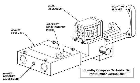
magnet assembly. A wide range of field strengths may be obtained to permit cancellation of the Earth's field at any location on the surface of the Earth by means of an adjustment screw . This adjustment is performed at the actual compass calibration site. The magnet assembly also provides an adjustment to compensate for misalignment of the aircraft with respect to a north-south line.
