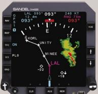
Drawing from our experience with thousands of compact integrated displays in service, we designed the SA4550 to do what no others can: Replace your electromechanical ADI with a modular electronic unit.
