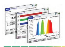
The PR-6xx design provides stand alone operation - no PC required. Menus are accessed via the on-board, 3.5" high resolution, full color touch screen LCD display and 5-way navigation keypad. Following a measurement, the PR-6xx displays **data** and color spectral graphs on the system display.
