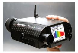
The patented Auto Sync<sup>®</sup> feature takes the worry out of accurately measuring high intensity, fast refreshing sources such as LCD's, PDP's, DLP Projectors, etc. by adjusting the detector exposure time to the source refresh rate. When enabled Auto Sync<sup>®</sup> insures that entire pulses are captured, improving the accuracy and repeatability of the measurements. The Sync rate of the source is displayed once a measurement is completed.
