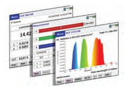
The PR-6xx design provides stand alone operation - no PC required. Menus are accessed via the on-board, 3.5" high resolution, full color touch screen LCD display and 5-way navigation keypad. Following a measurement, the PR-6xx displays **data and color spectral graphs on the system display.**
