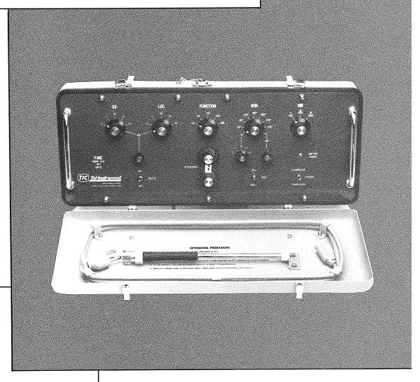
The Tel-Instrument Type T-30C Ramp Test Set is designed to meet the requirements of ICAO Annex 10 Category III specifications for one-man cockpit checkout of VOR, ILS, and MB receiving equipments. It can also be used to ground check flight director and autopilot systems.
