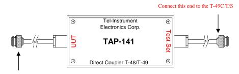
Connect this end to the Unit Under Test (UUT).
