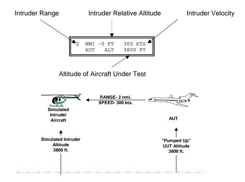
When utilizing the **+3500/-3500** Intruder Selection. The T-49C altitude will also increase or decrease (dependent on offset selected) altitude to intercept the Aircraft Under Test altitude. When the altitude and range converge, the test will reverse back out to the 14 nmi. initial range.
