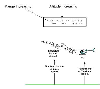
9. When you are unable to observe the simulated target on the TCAS display, reposition the TCAS directional Antenna to a different location. Observe that there are no obstructions between the Test Set and the AUT TCAS Antenna. If no display is still present, place the **TCAS/HI-XPDR/TCAS/LO** switch to the **HI** position.
