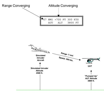
Once the Intruder Simulation reaches **0**, the simulation will reverse direction and return back to 14 nmi.
