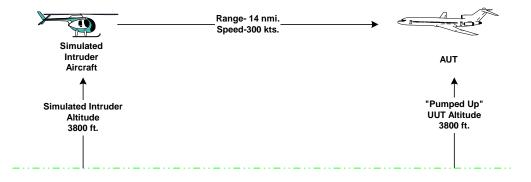
The Scenario will run from 14 nmi. to 0 nmi. and return back to 14 nmi. It will continue this cycle until another scenario is selected, the Test Set is turned "*OFF*" or times out.
