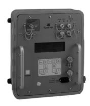
The TCAS-201 simulates the airborne environment necessary for verification/certification of TCAS installations
