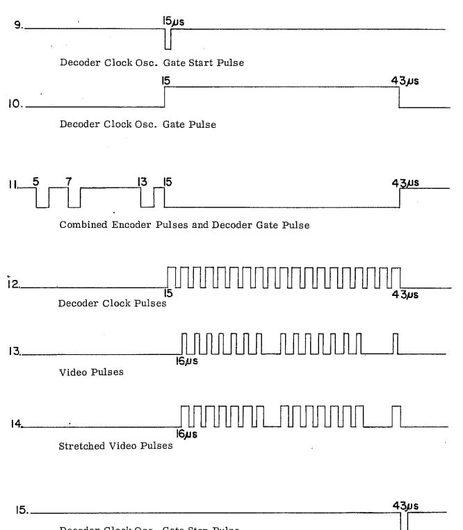
Decoder Clock Osc. Gate Stop Pulse
