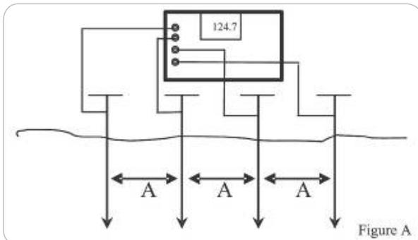
Two and three wire configurations can be used when measuring grounding effectiveness of existing ground rods and other grounding systems. In the four wire mode, the R1L-C measures soil resistivity over areas where the test rods can be placed as close as desired and up to 150 ft apart (see **Figure A**: an example of 4 wire soil resistivity measurement). Using a resistivity chart or simple formula, the ohmic reading is converted to a soil resistivity measurement in ohm-cm.
