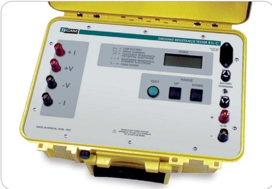
The Model R1L-C is a series of portable ground resistance ohmmeters designed to measure grounding system resistance, as well as soil resistivity, over ranges from milliohms to 20K $\Omega$  full scale. The R1L-C is capable of Wenner, Fall of Potential, 62% methods as well as bond and continuity measurements. Two, three and four point measurements are standard for this instrument.
