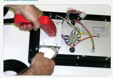
Shown left, The HTP-101A four-wire Kelvin probes are molded with a conductive additive to prevent the buildup of dangerous static electricity. They are also wired with 8 feet of #12 AWG cable and contain two stainless steel spring loaded pins that rotate as they are depressed to punch through corrosion and coatings. The pins are 0.158 in diameter and the pin center to pin center is 0.5 in (1.27 cm).
