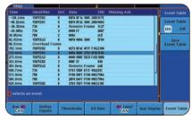
Packet decode table showing decoded Identifier, DLC, Data and CRC for every CAN packet in a long acquisition.
