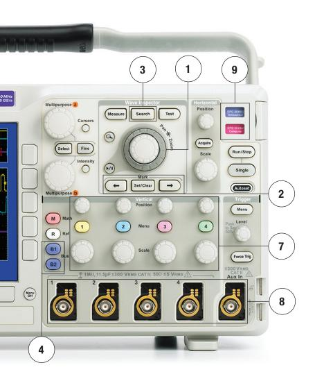
7 Vertical Controls – Knob-per- channel vertical controls provide simple and intuitive operation. No longer do you need to share one set of vertical controls across all four channels!
