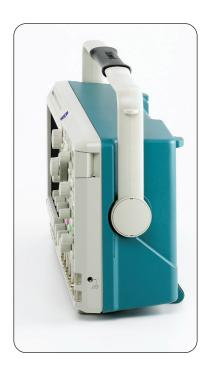
Only 5.4 in. Deep! – Despite the impressive performance, big display, and knob-per-channel controls, the DPO3000 Series is only 5.4 in. deep, saving you valuable space on your test bench.
