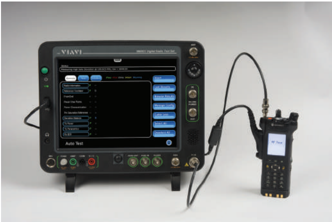
The 8800SX Auto-Test Setup
