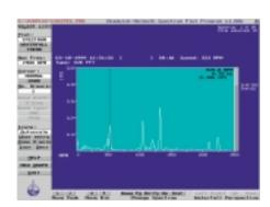
Spectral Plot lets you integrate and differentiate into any units... mils, IPS, g's, etc.
