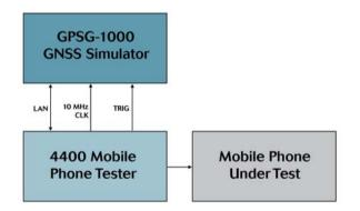
The 4400 utilizes the three file types, which are in a time stamped format, for creating assistance data that is sent to the phone under test upon request. The 4400, via the Ethernet interface, can arm the GPSG-1000 simulation and provide a hardware trigger of the simulation. The GPSG-1000 external 10 MHz clock is provided by the 4400, allowing the synchronization of the RF simulation with the data used in the simulation, stored in the 4400 memory.
