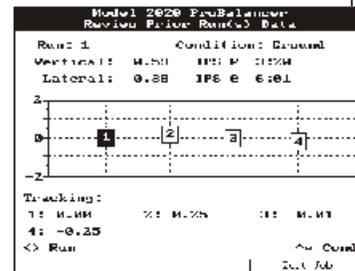
Each review screen contains all the information required to make adjustments to your job. The run number, condition, vibration amplitude/clock angle, and blade tracking information are recorded and readily available for viewing, printing, or storage with only a few keystrokes.
