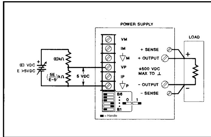
Figure 3-9. Optional Voltage Divider for Program Source
