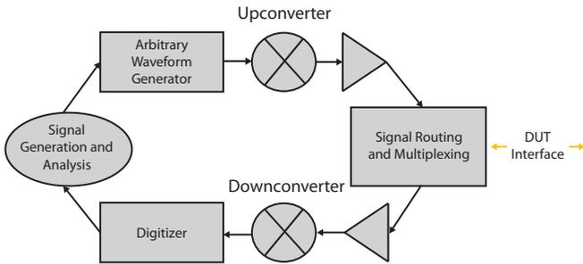
Figure 7. System architecture
