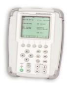
The IFR 4000 Navigational Communications Flightline Test Set verifies the operation and installation of ILS, VOR and Marker Beacon receivers and VHF AM/FM and UHF AM transceivers. The IFR 4000 with its lightweight size (under 8 lbs.), long run time battery (8 hrs) and ergonomic design will provide the user with the most portable navigational communications ramp test set on the market today.
