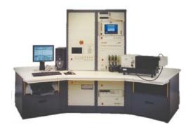
The Aeroflex IRIS® 2000 is a modular general purpose Automatic Test Equipment (ATE) system capable of testing a wide variety of avionics Line Replaceable Units (LRU). The IRIS® 2000 is the only ATE that combines the testing of RF, analog and digital LRU's in one ATE system.
