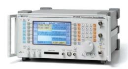
The 2948B Low Noise Communications Service Monitor with Option 25 offers an impressive range of features for the aircraft and avionics maintenance industry. The dedicated 2948B provides signals for testing the following: ILS receivers for localizer including identification, glideslope and markers; VOR beacon receivers with identification; SELCAL selective calling receivers.
