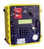
The IFF-701Ti is an organizational level/1st Line, portable battery operated test set for testing IFF transponders and interrogators installed in airborne, naval or land based platforms. The IFF-701Ti may also be used at an intermediate level/2nd Line.
