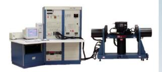
The IRS 1200 is an inertial reference test system used to test Honeywell Air Data Inertial Reference Units (ADIRU) and Inertial Reference Units (IRU) of air transport, commuter and business aircraft, as well as cockpit control panels and system display units. With the fully-automated configuration of the IRS 1200, an operator can initiate multiple NAV runs and allow the ATE to run overnight with no intervention. The system can be configured for the customer's fleet.
