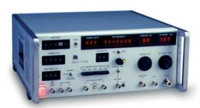
The RDX-7708 Test Set provides RF source and monitor for complete RF testing of ARINC 708 T/R (Transmitter/Receiver) units including wind shear variants. Transmitter power measurement is via a waveguide mounted RF power module. This method minimizes measurement errors due to RF coaxial cable loss variations.
