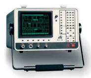
The MLS-800 is a microprocessor controlled simulator, designed to test airborne MLS angle receivers on the bench or verify system operation on the ramp. The parameters displayed on the MLS test menu are in accordance with the RTCA/DO-177 specifications and EUROCAE ED-53A.
