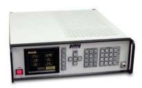
The NAV-2000R is the only generator needed to test ADF, Marker Beacon, VOR, LOC, Glideslope, HF, VHF and UHF COMM receivers. The NAV-2000R Signal Generator offers a frequency range of 150 kHz to 450 MHz, and is loaded with special avionic functions including the ability to produce Morse Code Ident in VOR, LOC and ADF modes; pulsed audio tones corresponding to the Marker Beacon selected; two-tone modulation; and SELCAL capability in COMM mode.
