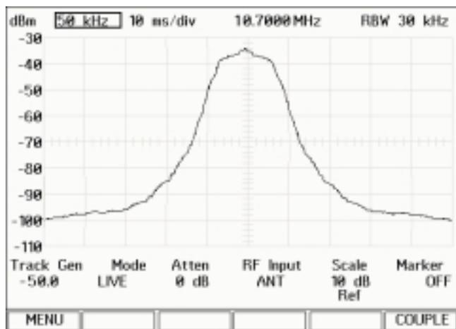
Figure 6.0 - IF After Alignment with Gain of 10 dB
