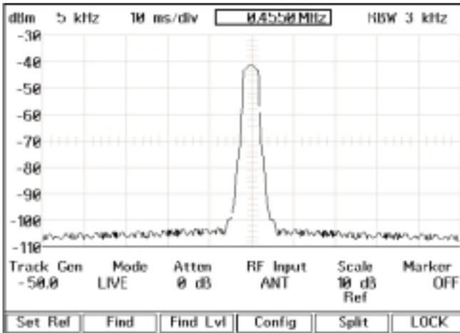
Figure 7.0 - Results of Changing the Span to 5 KHz/division
