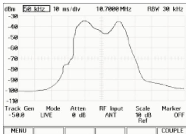
Figure 5.0 - First IF Display Indicating Alignment is Required
