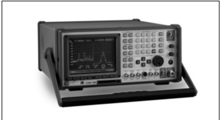
An improperly aligned IF stage can rob a receiver of important sensitivity - sometimes as much as 20 to 30 dB. The resulting loss of coverage (or increase in transmitter power to make up for it) will increase the cost of operating a radio system. However, by using the advanced features of the IFR COM-120B's tracking generator, your receiver can be kept in top working order.
