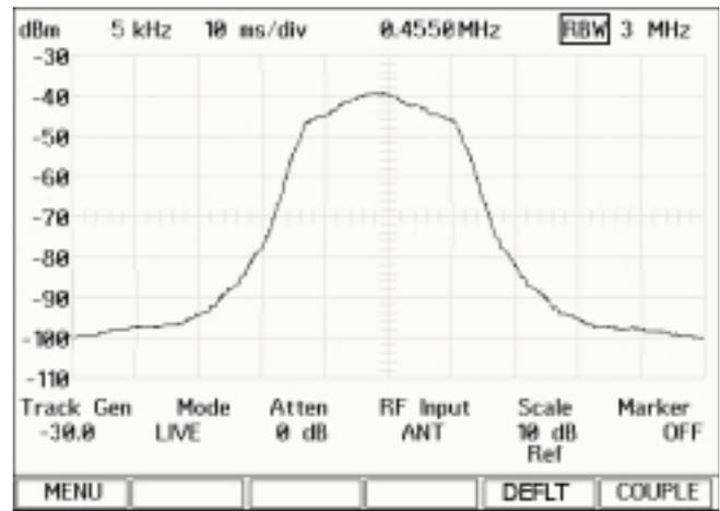
Figure 8.0 - Opening up the Resolution Bandwidth to 3 MHz
