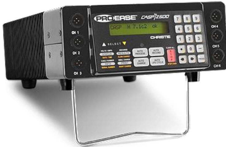
The CASP/2500H Universal Battery Support System performs all of the advanced battery support functions of the CASP/2000, but with expanded battery processing capabilities and the latest internal firmware. Functions include fast charge, slow charge, discharge, analyze, recondition and maintenance charge. Rated at up to 10 amps and 78 volts with six output channels, the CASP/2500H can process a wide variety of batteries automatically while generating detailed battery servicing reports via
