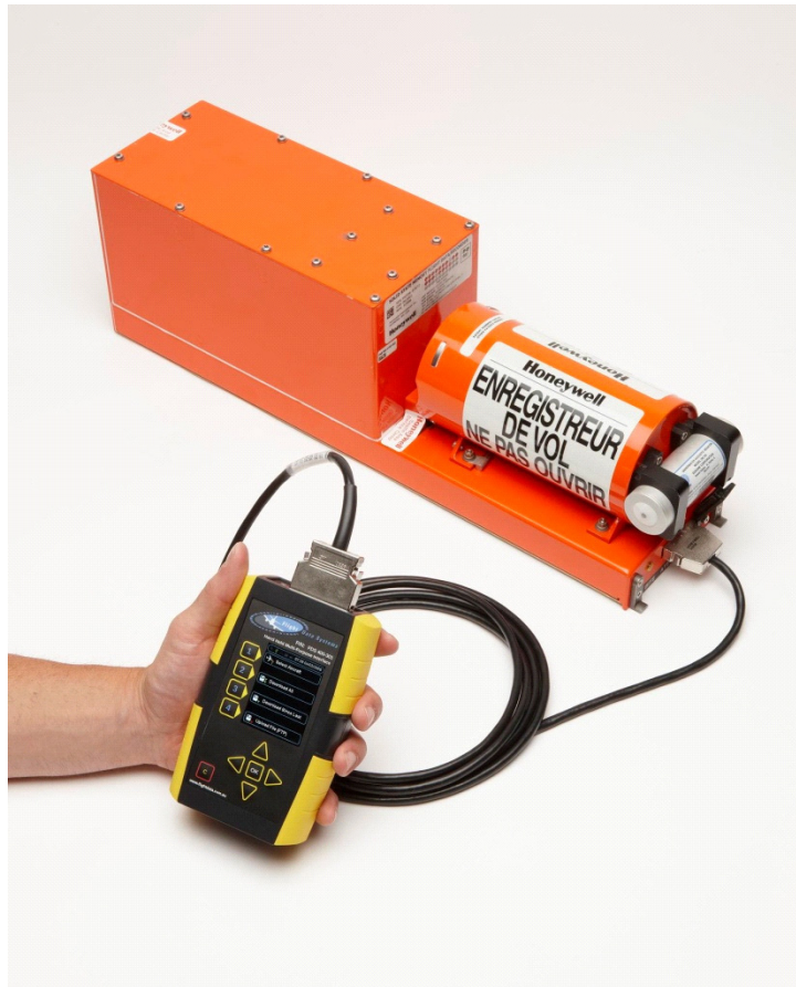
Figure 7.0 Connecting the HHMPI to the FDR or CVR
