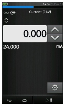
Figure 2-18 Source current on CH2 with internal loop power. (Range: 0 to 24 mA)
