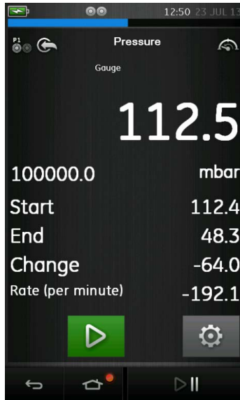
Figure 3-9 Leak Test Example
