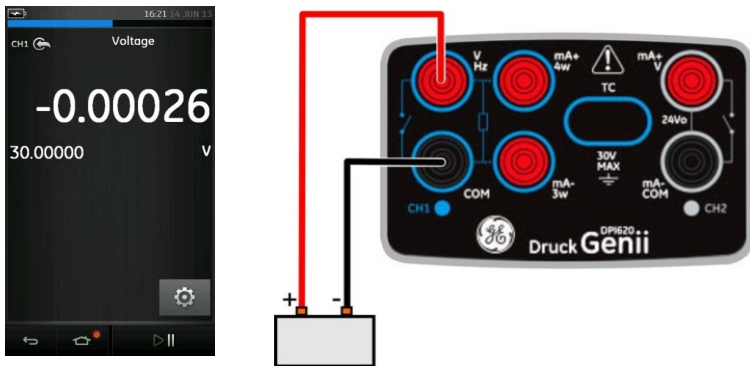
Figure 2-14 Measure DC Volts or DC mV on CH1. Range \pm 30 V
