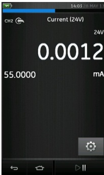
Figure 2-19 Measure current on CH2 with internal loop power (Range: \pm 55\text{mA} )
