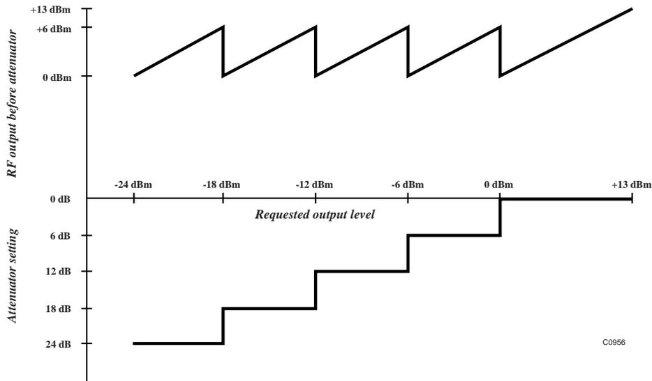
Fig. 3-1-35 Normal signal generator level control operation
