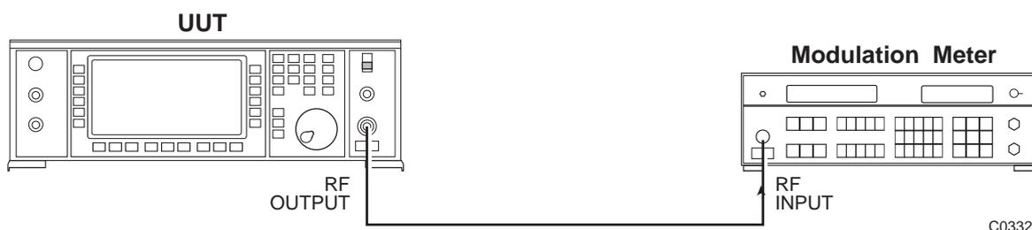
Fig. 5-1-9 Internal AM depth and distortion test set-up
