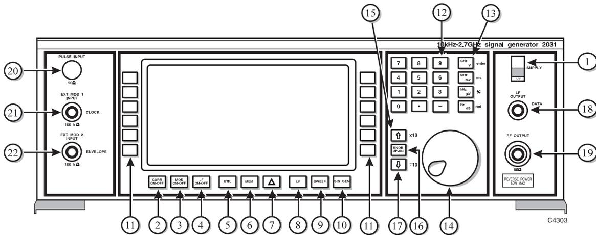
Fig. A-1 2031 series front panel with Option 005
