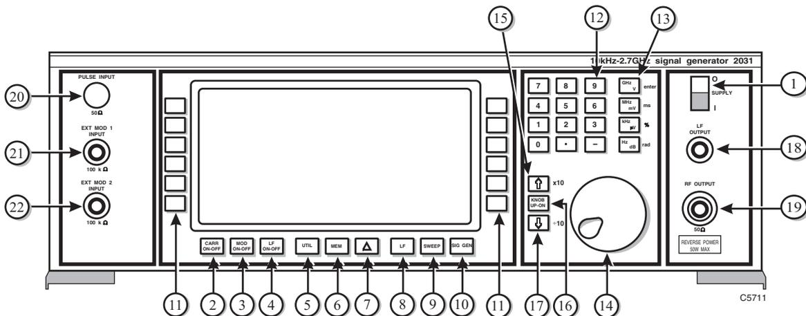
Fig. 3-1-1 2031 front panel
