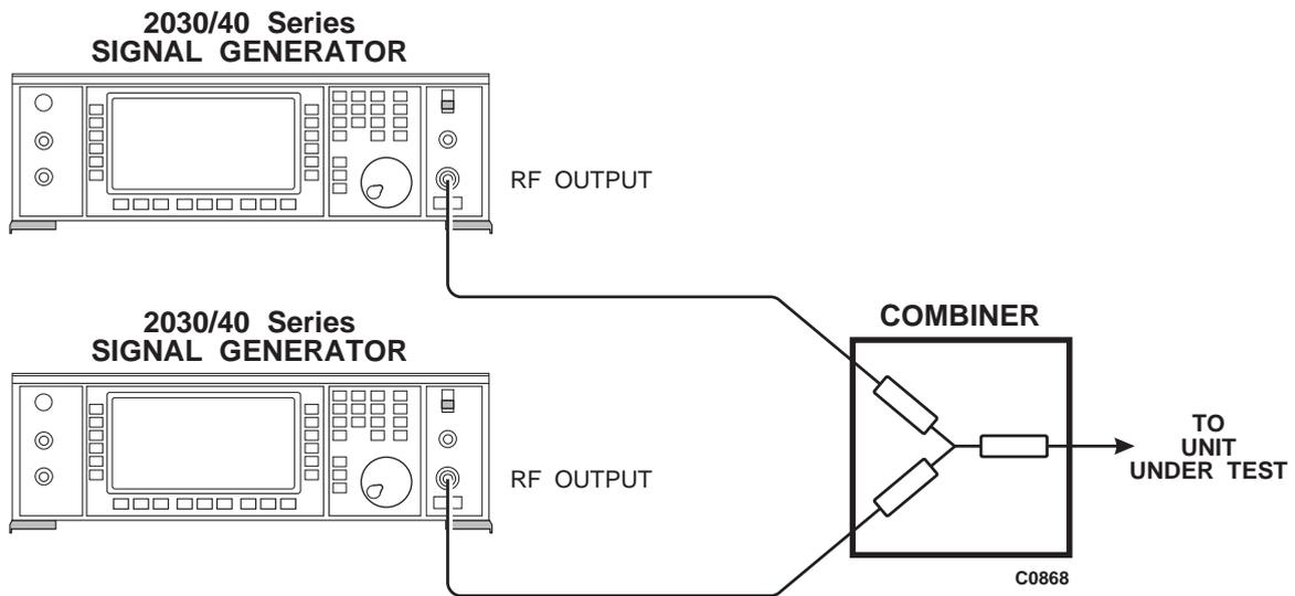
Fig. C-8 Two signal generator testing with a resistive combiner
