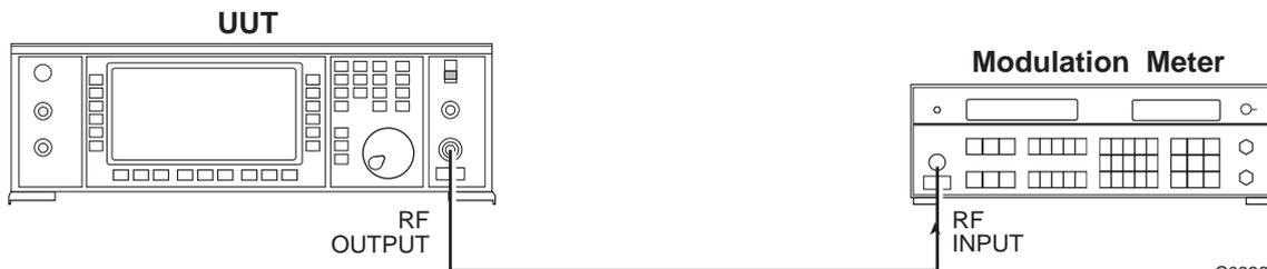
Fig. B-28 Accuracy of SDM signal path test set-up
