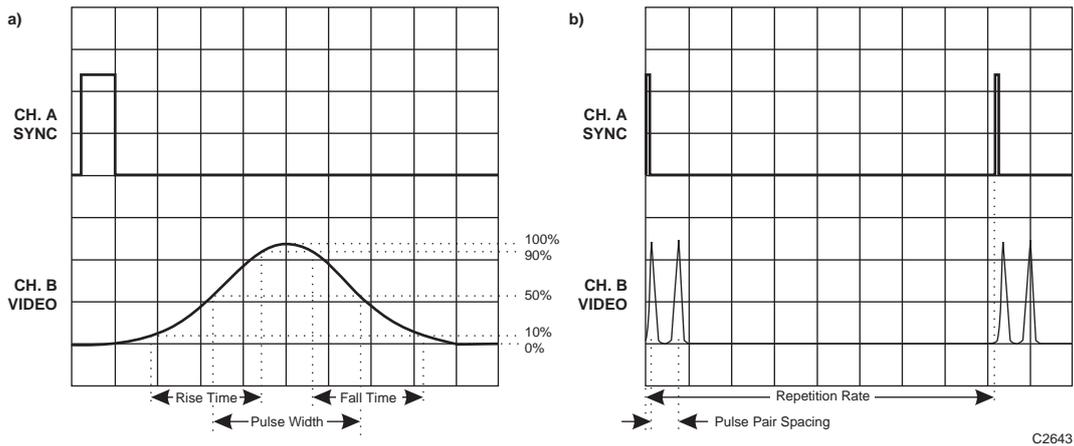
Fig. E-12 Oscilloscope traces for SYNC and VIDEO outputs
