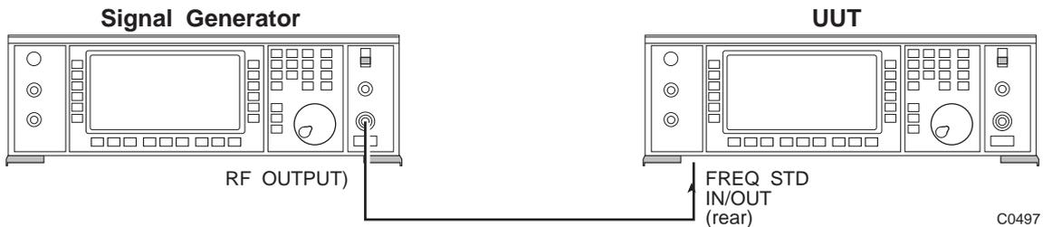
Fig. A-25 Frequency standard locking test set-up
