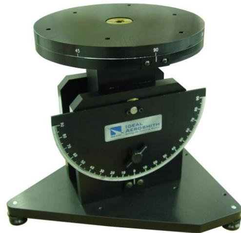
ball engages detents in the bottom of the tabletop, locking it into position for quick setup. The detents are located every 45°. Tables with optional engraved marks every 1° have detents every 15°. The tension is adjustable for the positioning detents on both the tabletop and the tilt axis.
