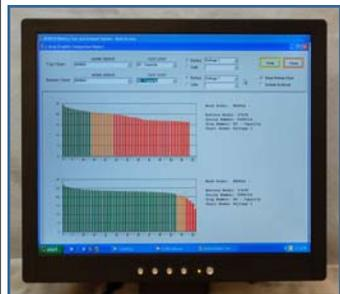
**BTAS16:** Computerized System for the acquisition of data from batteries under test.
