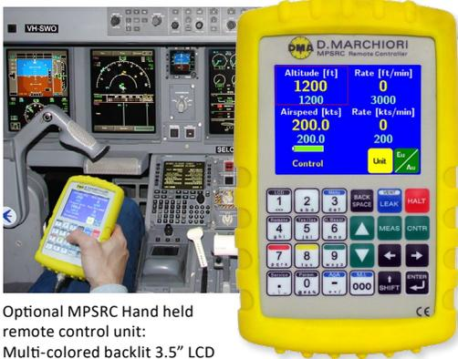
Optional MPSRC Hand held remote control unit: Multi-colored backlit 3.5" LCD touchscreen and keypad
