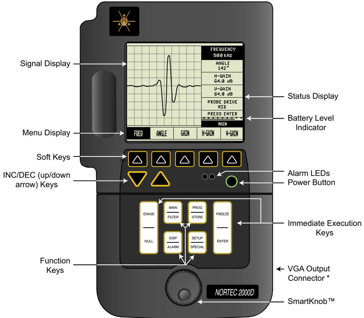
\* only available on 2000D+ models. This connector is only active when a color display is installed.
