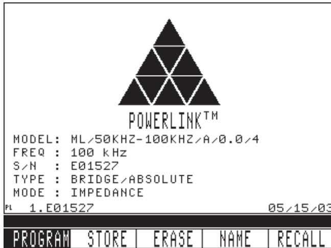
After the PowerLink™ screen appears, you can recall any existing program that has been saved in the program storage menu. By rotating the SmartKnob™ clockwise, the list of pre-stored programs and the date stored will appear at the bottom of the display.
