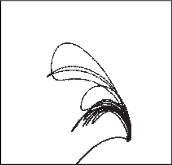
**Figure 4-3. Second Layer Crack Detection**
