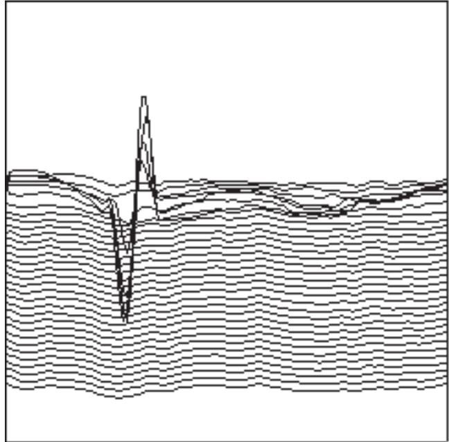
**Sample Defect in a Hole Standard**
