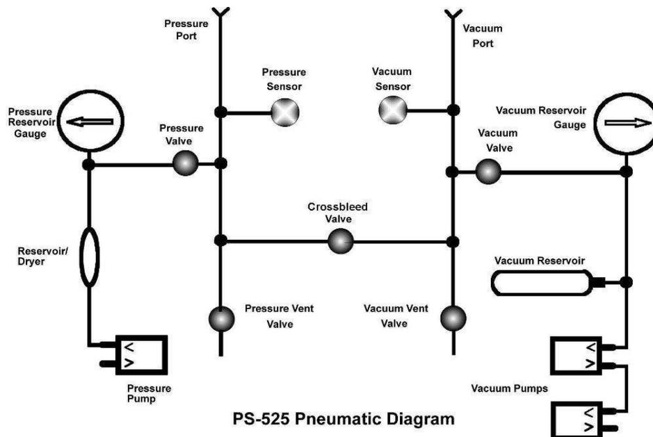
When the operator wishes to simulate an altitude, the Crossbleed, Vacuum, and Vacuum Vent valves are gently closed. The vacuum pump is then energized until sufficient vacuum is in the reservoir, as indicated on the Vacuum Reservoir Gauge. How much vacuum will be needed depends on the desired altitude, and is also affected by how long the tubing and lines are between the test box and the altimeter. **The vacuum and**
