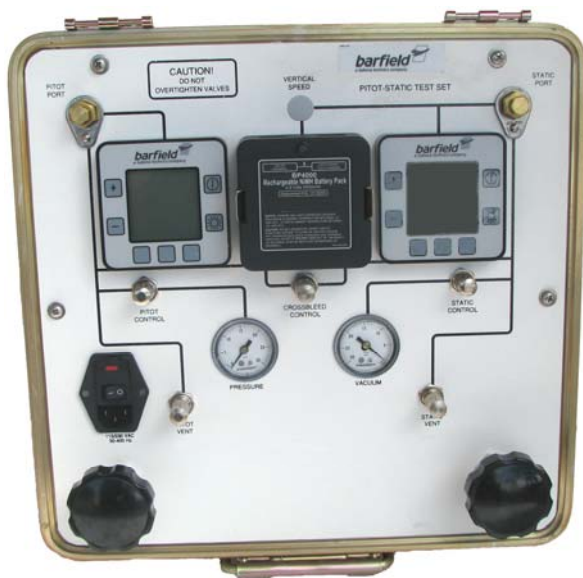
1811HA Test Set (P/N 101-00184-SERIES)
