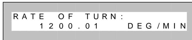
The Run Display must be active in order for the remote communications port to be active. The communications port cannot be used while an operator is inputting information on the front panel. The keypad can be disabled to prevent the operator from interrupting a test. (See KPE Command, Section 3.4)
