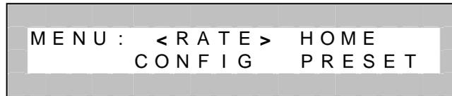
Pressing the increase or decrease key will toggle the <> among the four menu choices. Press the enter key after the selection has been made. If you wish to return to running the last rate at this time, press the Run/Menu key. If the Run/Menu key is not pressed, the table will return to the run display (zero rate) after approximately 10 seconds of inactivity. After this ten second period, the remote communications will be enabled.
