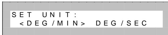
Press increase (decrease) key until desired unit is enclosed in <> and press enter. The desired units will now be set and the main menu will be displayed. The current unit system is always shown in the run display.
