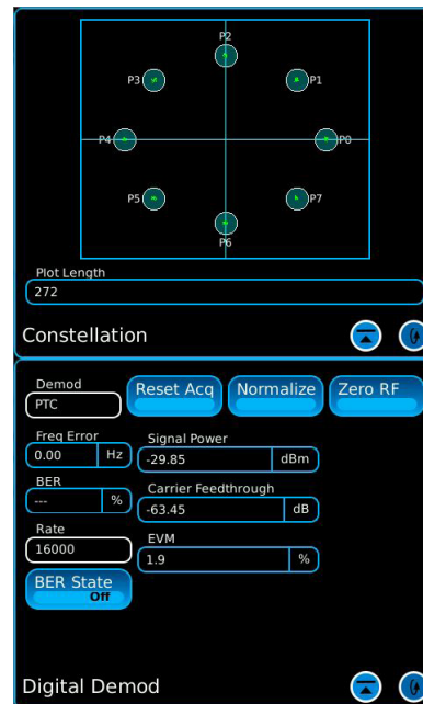
PTC Option Showing Digital Demod and Constellation
