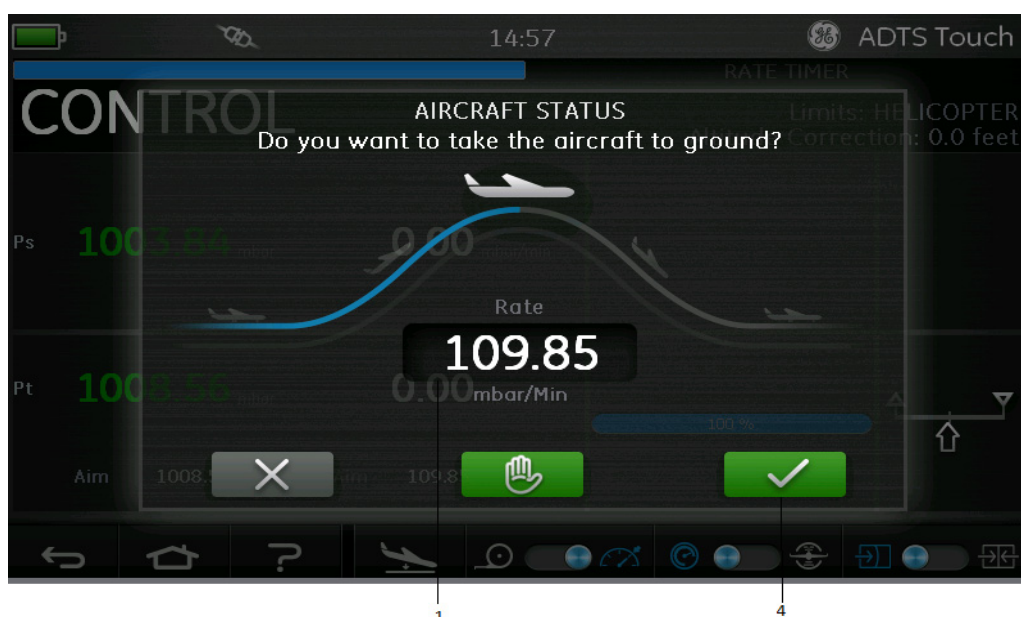
Figure 3-18: Go to ground main screen - Single Channel
