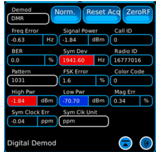
Meters with Color Pass/Fail Indicators
