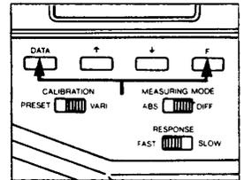
Set Y by pressing and holding **[F]** and pressing either **[↑]** or **[↓]** until the displayed value is equal to the desired value.
