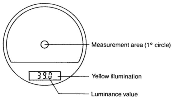
The measurement area and measured luminance value can be simultaneously confirmed in the viewfinder as shown in the figure above. The display is a digital liquid-crystal display (LCD) illuminated with a yellow LED.
