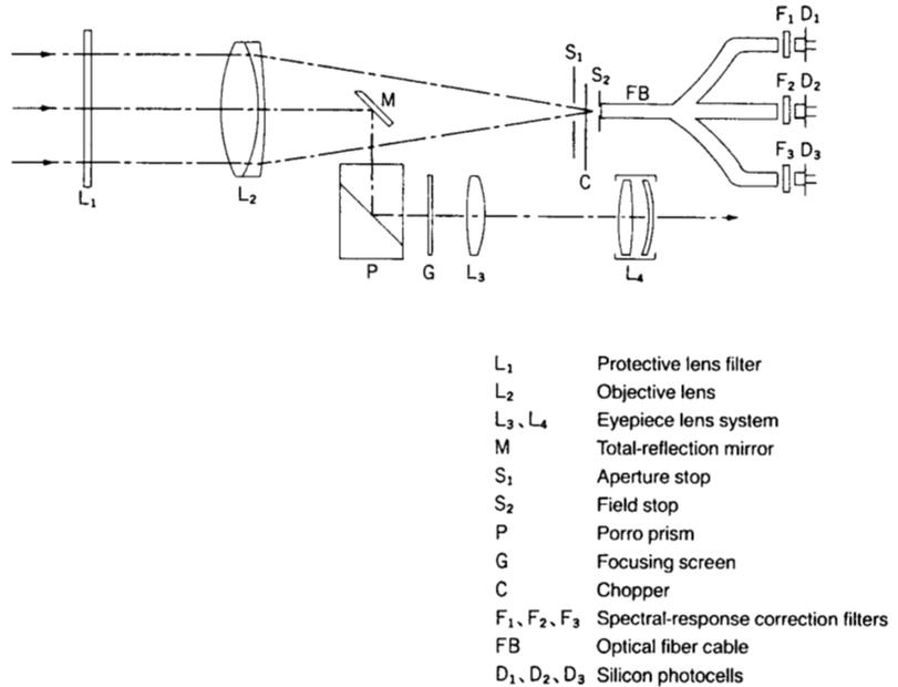
As shown in the above figure, Konica Minolta optical technology is used to realize a handheld metering system. Use of an in-viewfinder display also enables simultaneous confirmation of the measurement area and measured luminance value, resulting in a more compact, lightweight chroma meter. The endface of the optical fiber cable is located where the objective lens focuses, as are the display and focusing screen with circular measurement-area indication.
