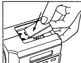
4. Replace the cover by realigning it and sliding it towards the meter body until it snaps securely into place.
