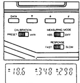
12. To store the values for Yxy in memory and complete calibration, slide the CALIBRATION selector switch from **VARI** to **PRESET** (if not set to **PRESET** in step 2), press and hold **[F]**, then slide the switch back to **VARI**. The external display will read "CAL" for a moment as the Yxy values are stored and the meter automatically adjusts its calibration, then the display will revert to the Yxy values.
