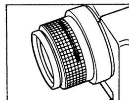
5. Pull the measuring trigger and hold it in until the luminance value (Y) appears in the viewfinder display. Yxy values will appear in the external display.
