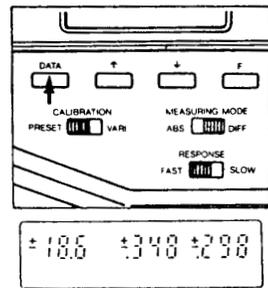
7. Slide the MEASURING MODE selector switch to **ABS**.
