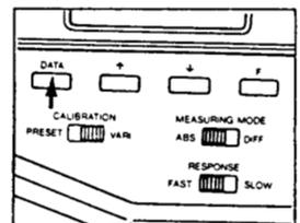
17. Slide the CALIBRATION selector switch from **VARI** to **PRESET**, press and hold **[F]**, then slide the switch back to **VARI**. The external display will read "CAL" for a moment as the Yxy values are stored and the meter automatically adjusts its calibration, then the external display revert to the Yxy values.
