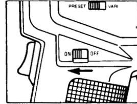
2. Set the MEASURING MODE selector switch to **ABS.** and check that the CALIBRATION, RESPONSE speed, and luminance-unit selector switches are set to the desired positions.
