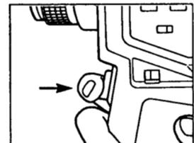
5. Store the values measured in step 4 by pressing and holding **F** and sliding the MEASURING MODE selector switch to **DIFF**. The external display will read "CAL" for a moment as the target values are stored, then revert to the previous display. The stored data will remain in memory until changed or cleared by user.
