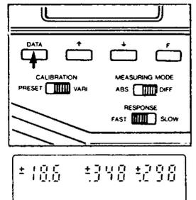
9. To store the values set for Yxy, slide the MEASURING MODE selector switch from **DIFF.** to **ABS.** Press and hold **[F]**, and slide the switch back to **DIFF.** The display will read “CAL” for a moment as the reference values are stored, then revert to the previous display. The stores data will remain in memory until cleared or changed by user.
