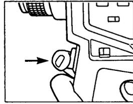
5. Store the value measured in step 4 by pressing and holding **F** and sliding the MEASURING MODE selector switch to **DIFF**.
