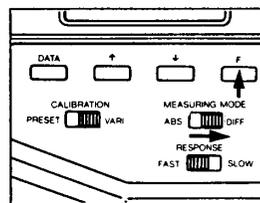
Press and hold **[F]** and press **[DATA]**. To indicate that the data has been correctly stored, the display will show all values as zero.
