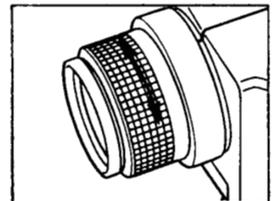
15. Pull the measuring trigger and hold it in until the luminance value (Y) appears in the viewfinder display. Yxy values will appear in the external display.
