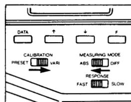
2. Press **[DATA]**. The previously stored calibration data for the user's standard will appear in the display. "±" will appear before each figure.
