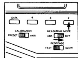
Press and hold **[F]** and press **[DATA]**. To indicate that the data has been correctly stored, the display will show all values as zero.
