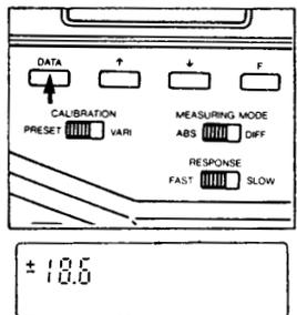
Set Y by pressing and holding **[ F ]** and pressing either **[ ↑ ]** or **[ ↓ ]** until the displayed value matches the desired value.
