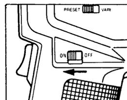
3. Set the CALIBRATION selector switch to **PRESET** and the MEASURING MODE selector switch to **ABS**. Check that RESPONSE speed and luminance-unit selector switches are at the desired positions.
