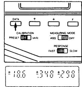
8. Slide the MEASURING MODE selector switch to **ABS**.
