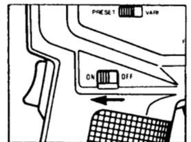
2. Set the CALIBRATION selector switch to **PRESET** and the MEASURING MODE selector switch to **ABS**. Check that RESPONSE speed and luminance-unit selector switches are at the desired positions.
