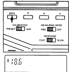
Set Y by pressing and holding **F** and pressing either **↑** or **↓** until the displayed value matches the standard value for the white plate being used. Values for CIE Standard Illuminants A, C, and D<sub>65</sub> are listed on the inside cover of White Calibration Plate CS-A20; values for CIE Standard Illuminant C and D<sub>65</sub> are listed on the inside cover of White Calibration Plate CS-A21.
