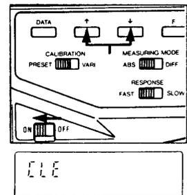
2. While pressing
