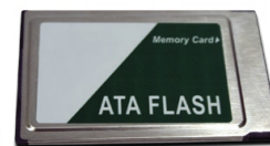
High-capacity PC card (PCMCIA) allows for storage of data from multiple aircraft flights
