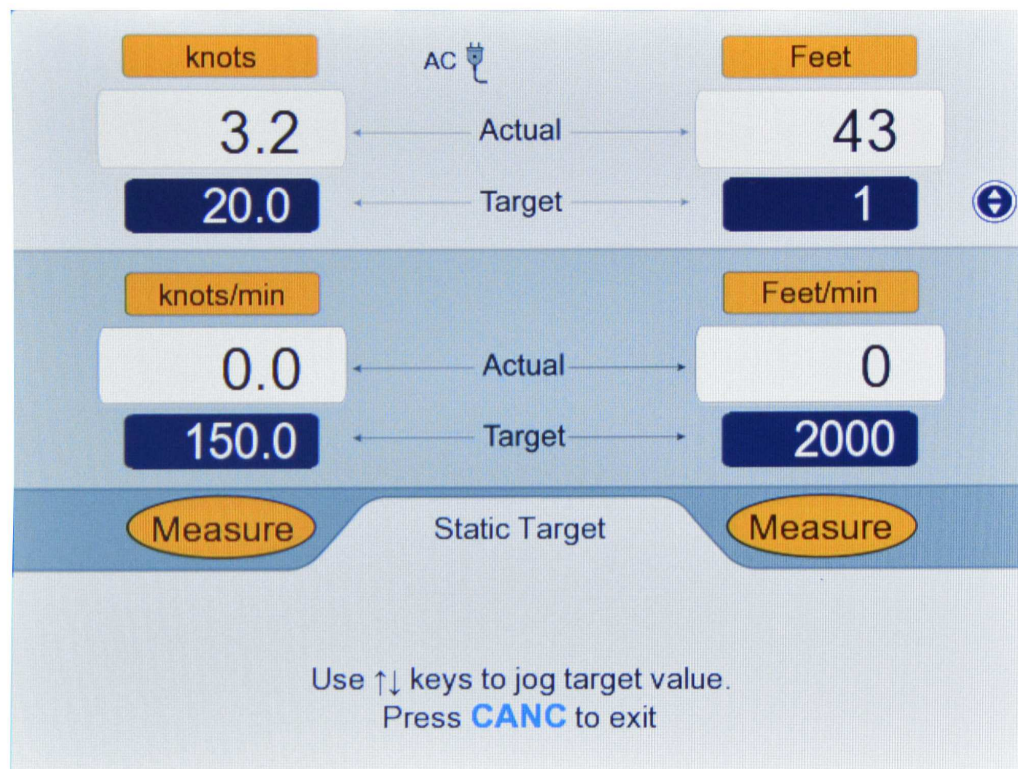
Figure 3.10 : Jog the Static Target value
