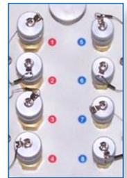
This multiple line switching permits fast and safe isolation of the lines to isolate leaking channels. Control is possible from any of the local or remote user interfaces. Combinations of line switching are also possible for numerous fault finding routines.
