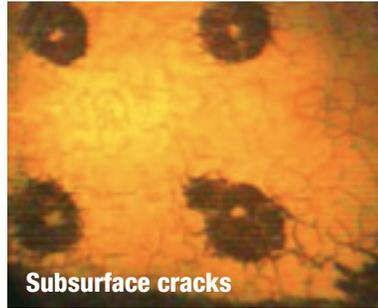
This is a third layer crack image that is 0.084" from the surface. The frequency has been set to 5 kHz resulting in a more diffuse image. Since surface cracks will also be visible, it is important that the inspector perform a high frequency scan first and mark surface defects. When the frequency is lowered, new crack images are subsurface defects.
