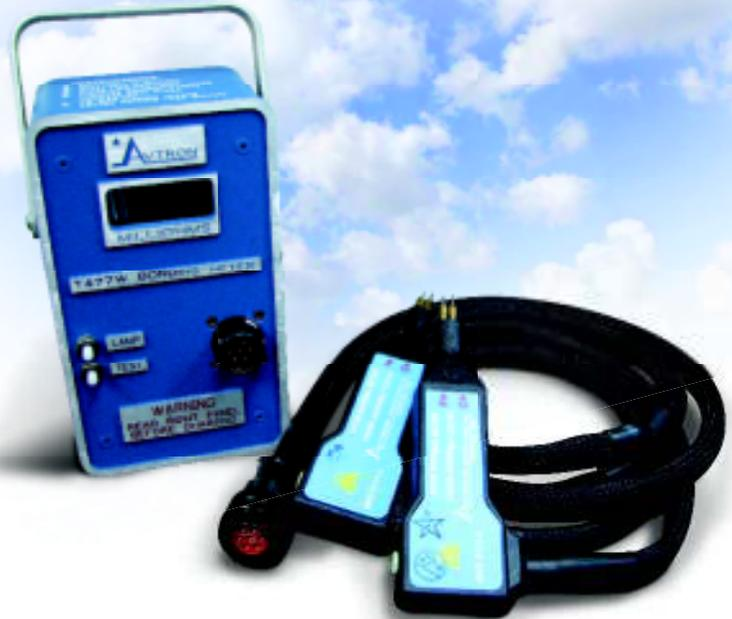
The low voltage and current output will not cause ignition of flammable gas, as certified by Underwriters Laboratories per UL 913, standard entitled "Intrinsically Safe Apparatus and Associated Apparatus, for use in Class I, II, and III, Division I Hazardous Installation." The meter is approved for use in Class I, Groups A, B, C, or D, which includes hydrogen and gasoline flammable vapors.
