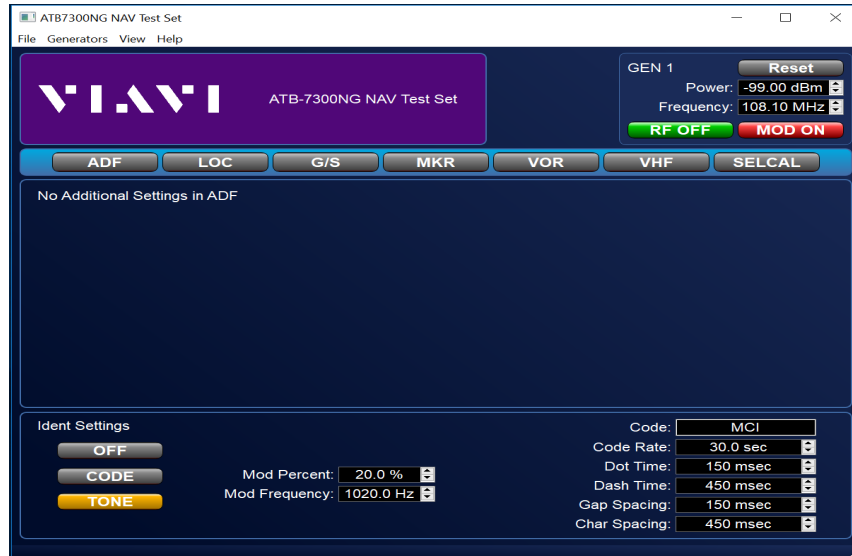
Figure 2-9 ADF Generator Instrument
