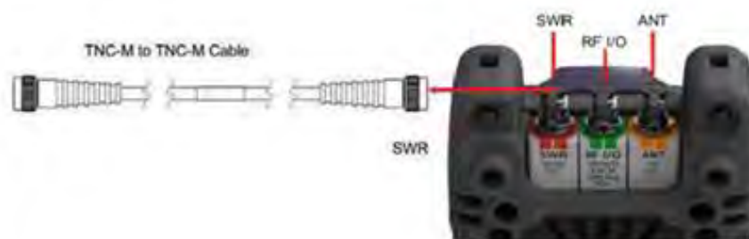
Figure 18: VSWR Calibration Setup Diagram
